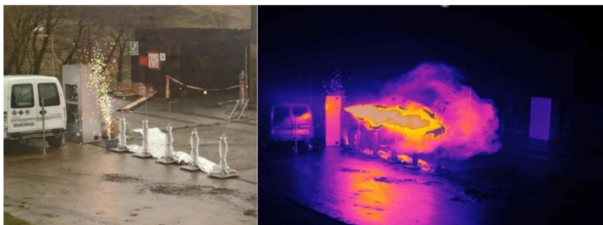
Figure 15 - Standard (left) and IR image of a jet flame (right)
